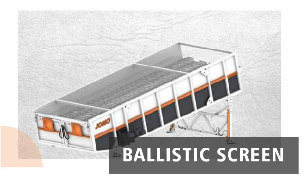
Adopting the imported German crankshaft mechanism transmission, ballistic screen can sort the materials into three categories and bounce off the materials attached to the package to achieve an unparalleled sorting effect.
