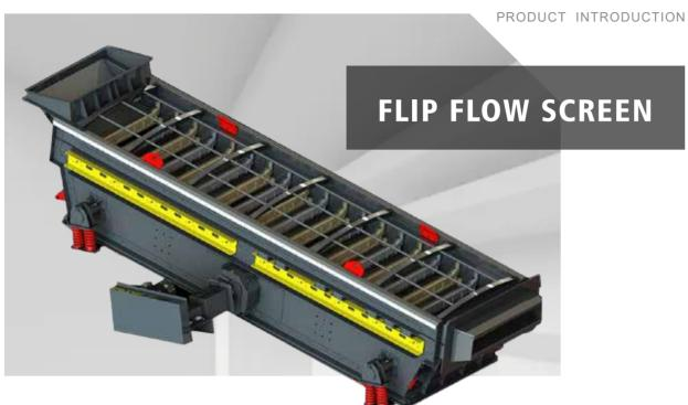
The Flip-Flow action stretches and slackens the screen mats very quickly. This action prevents build-up of fines material in corners or pegging in the screen mat apertures. The JONO Flip-Flow can screen to very small particle sizes because of this unique action. It is used in dry screening construction waste, crushed stone, sand, compost, wood chips, recycled glass and carpet fibres, slag and recycled electronic parts to name only a few applications.
