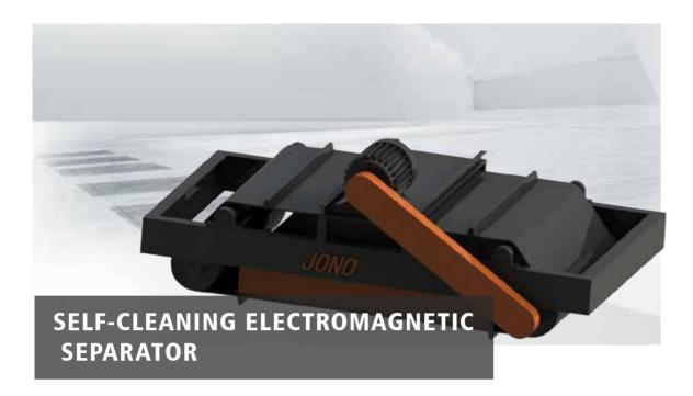
RCDD series of dry-type magnetic separator is a kind of electromagnetic equipment to clean up ferrous metal form bulk non-magnetic materials and is used to automatically remove 0.1-25kg of magnetic material from non-magnetic materials.
