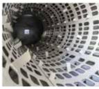
rial drops through the screen holes, the big sized material will be discharged at the discharging chute at the end. This rotation can make sure the material go through enough holes to greatly optimize the separation effect.
